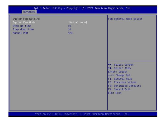
Step up time: The amount of time fan takes to increase its value by one step. (Units are intervals of 0.1 second).  $10 \times 0.1 \text{ sec} = 1 \text{ sec}$  as default.
